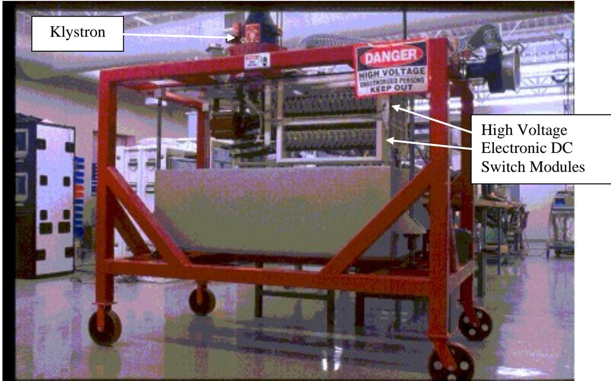
**Radtec TDR 43-250 DC Switch Modulator Test Stand**
