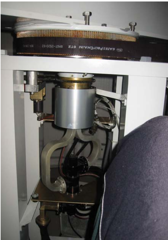
Below: Antenna azimuth drive showing slip rings and dual polarity waveguide feed.
