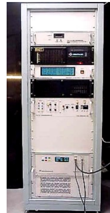
RDR-250GC 250 kW C-Band Coaxial Magnetron Radar
