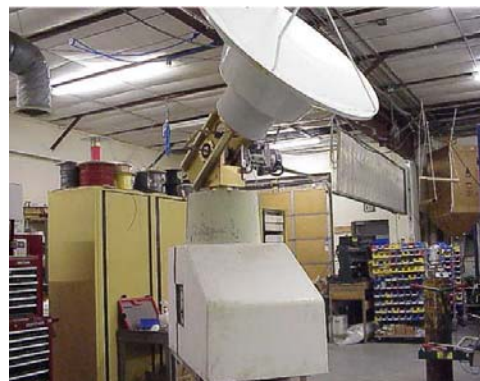
RDR-50GX 50 kW X-band Radar for a military project requirement
