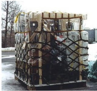
Tactical weather radar system- Complete fully coherent C-band system, including antenna and tower, packaged on one standard air freight pallet, fits in C130 type aircraft. Setup by 2 person crew with no additional equipment. Only shelter and electrical power required.
