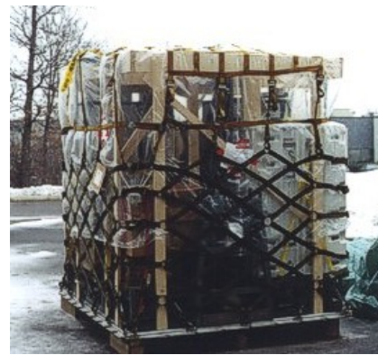
Complete, transportable TDR 2070C, including antenna, self extending tower, and workstations packed on one airfreight pallet.
