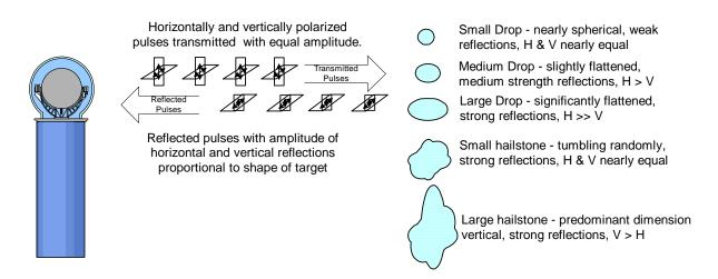
Research to date indicates that dual polarity radars can routinely provide rainfall measurements that are within  $\pm 10\%$  to  $\pm 15\%$  of the "ground truth" from rain gauges.
