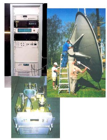
**Better Technology** - Coaxial magnetron, solid state IGBT modulator, and integrated low noise receiver front end, provision for future capabilities such dual polarity operation.
