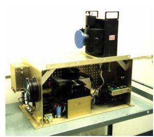
1 MW S-band transmitter module with automatic power-up sequence, automatic duty cycle limit protection, and BITE features.
