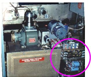
Solid State Modulator Upgrade Applicable To Many Existing Thyratron Radars
