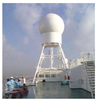
This installation provides a full set of Doppler weather radar data products, including volume scan products, whose quality and accuracy is comparable to the best shore-based systems.
